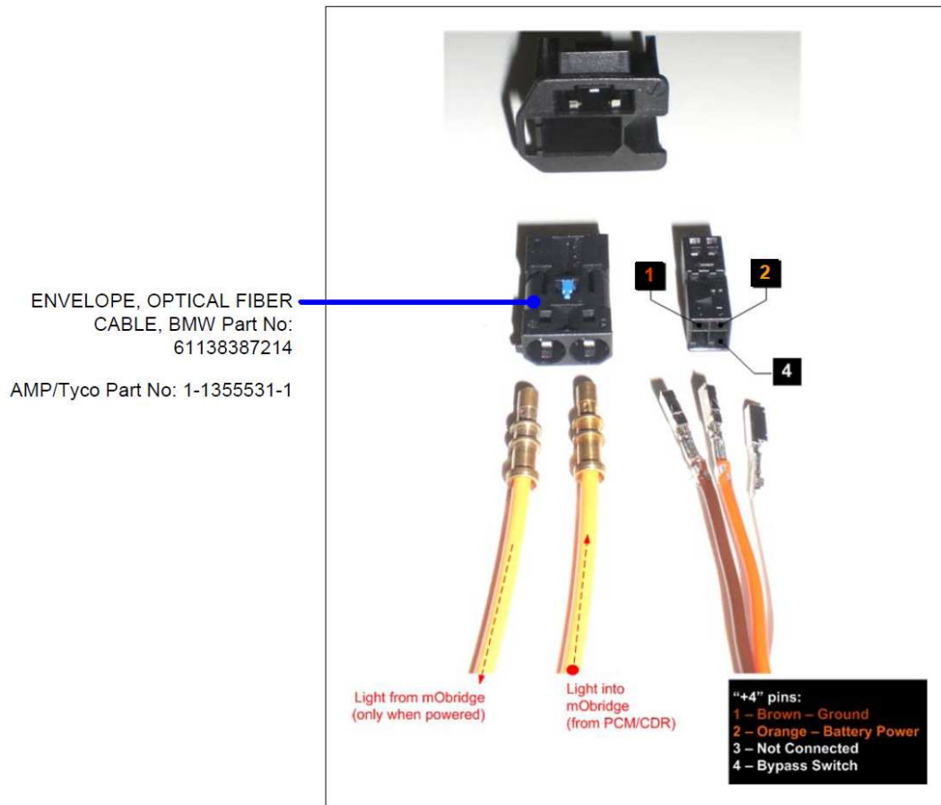
Figure 5 Fully disassembled mObridge wiring assembly
